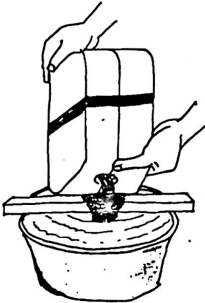
FIGURE 4. Draining the Mold
