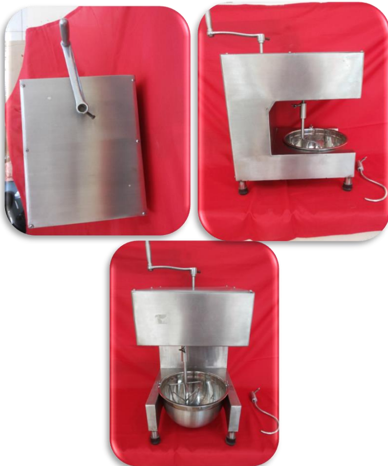
Figure 7. Hand-Operated Mixer for Batter, Dough, and Egg White Foam Top View, Side View, and Front View Pictorial Representation
