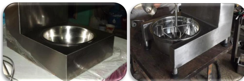
Figure 5. Hand-Operated Mixer for Batter, Dough, and Egg White Foam Pictorial Representation Before and After Enhancing
