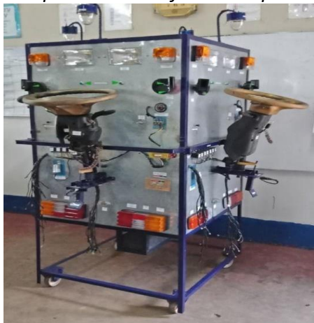
Prospective view of vertical quadrant auto-electrical mock-up
