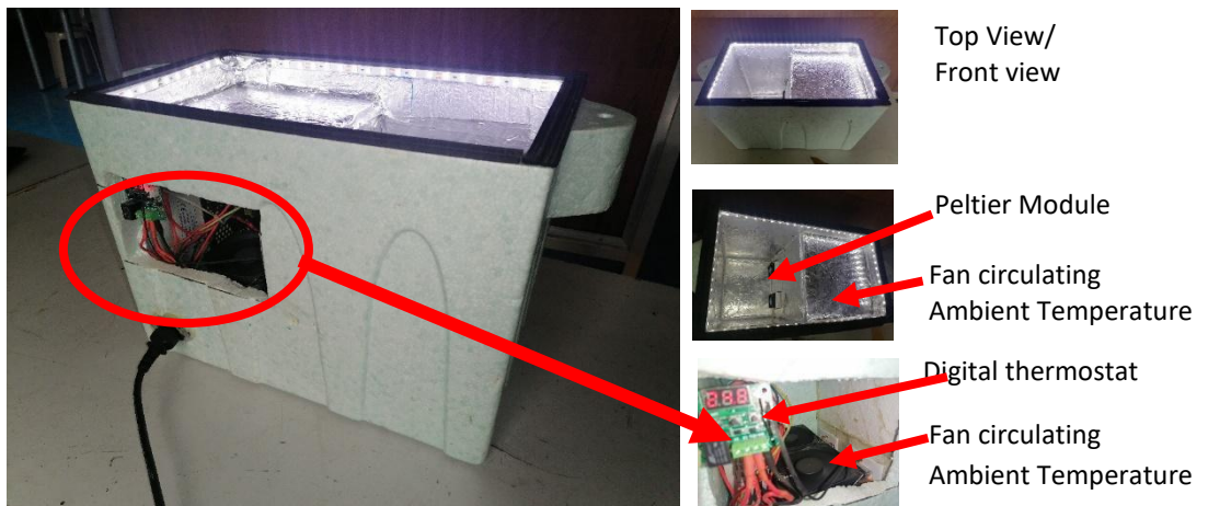
Figure 5 Main body of refrigeration chamber
